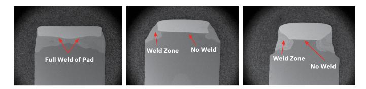
In these cross sections of the electrodes, note that the welding of the Bosch spark plug supports the entire iridium pad. In the other plugs, the welded zone is only on the edges of the precious metal pins. This complete weld, ensures the precious metal pin has the strongest connection possible to the base material and will not separate even in the most demanding applications.
